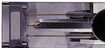
Nozzle is sealed by two cylinders
